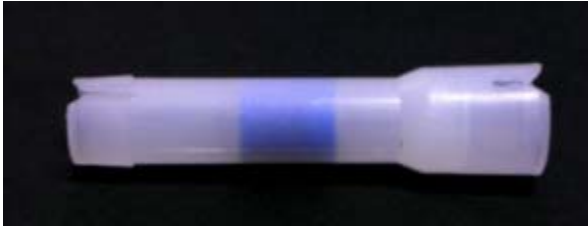
Fuse-holder with the delay inserted.
